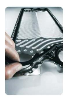
One of the main arguments for using PHEs instead of BPHEs is that PHEs can be taken apart and thoroughly cleaned. However, the process of chemically cleaning a PHE can be very expensive. The gaskets have to be removed prior to cleaning, and if they are glued to the plates (as many types of gaskets are), they have to be replaced at high cost with new ones after cleaning.
