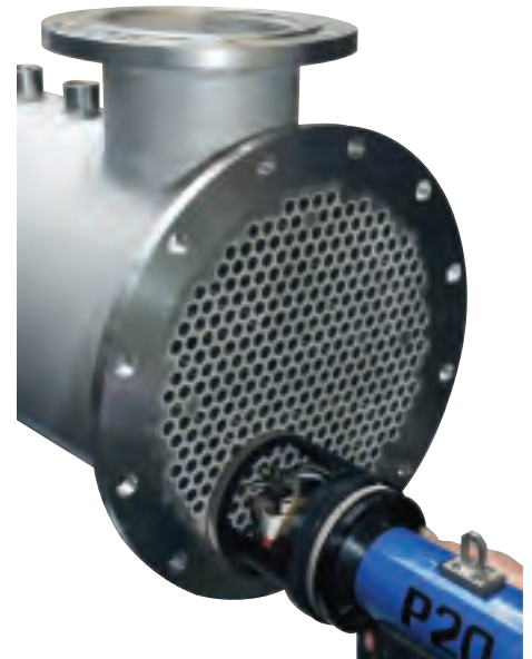
Automated tube end welding and 100% inspection
